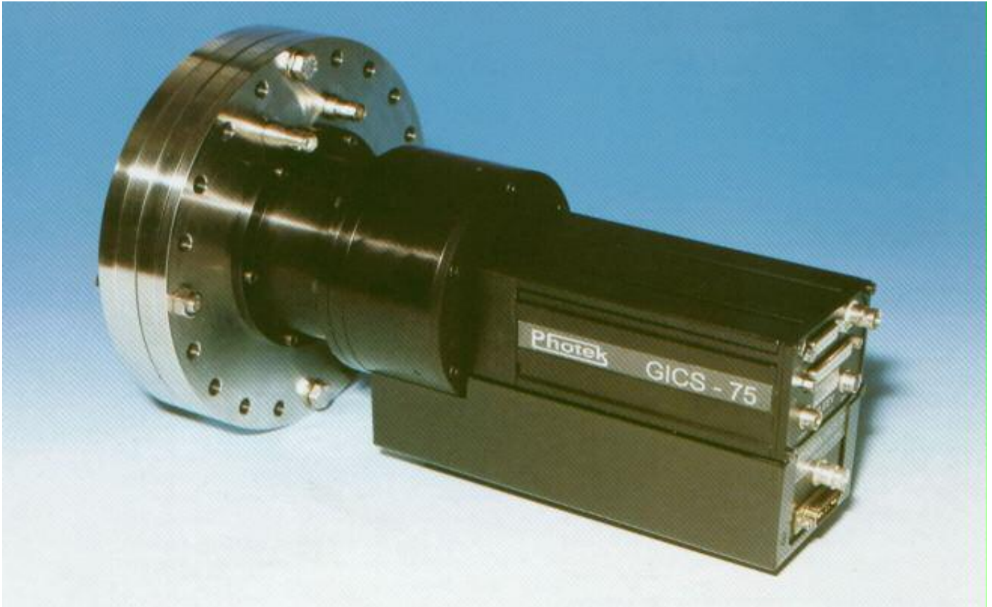
GICS-75 – A 75 mm active diameter MCP detector fibre optically coupled to a Photon Counting ICCD Camera with 5 ns gating and synchronous 512 x 512 CCD and custom image processing software
