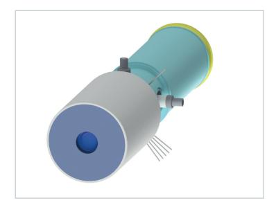
Streak tubes are used for the study of ultra fast optical phenomena and specifically measure the variation in light intensity as a function of time.
