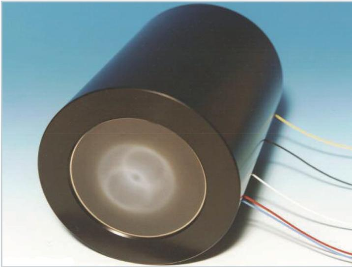
**Demagnifiers are electrostatic focusing devices used for the detection of light particles where reduction in image size is required. The Photek Demagnifiers are available with either a 47 mm, 80 mm, or 150 mm diameter input window. They have high dynamic range, high resolution and are an efficient alternative to fibre optic tapers.**
